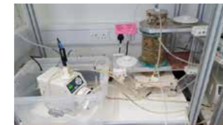
Advanced Anaerobic Digester including a pH feedback loop, and liquid recirculation.
